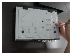
④ fix the screw of hard disk
