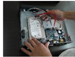
③ connect hard disk and mother board
