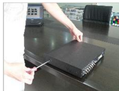
① Remove the screws on both sides of shell
